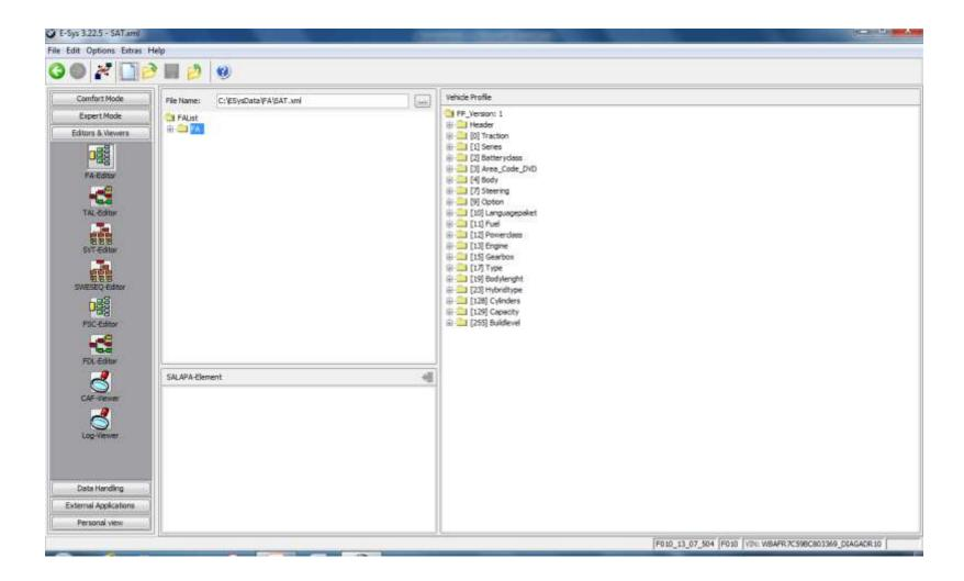
Expand the FAList folder system on left until SALAPA-Element is visible. Click on SALAPA-Element to select it.
