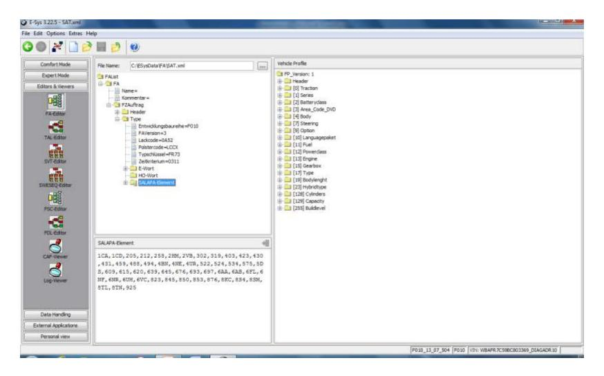
Delete or add Elements directly into the bottom window. In this example 205 is highlighted and will be deleted. The syntax is alpha-numeric and commas only, no spaces.
