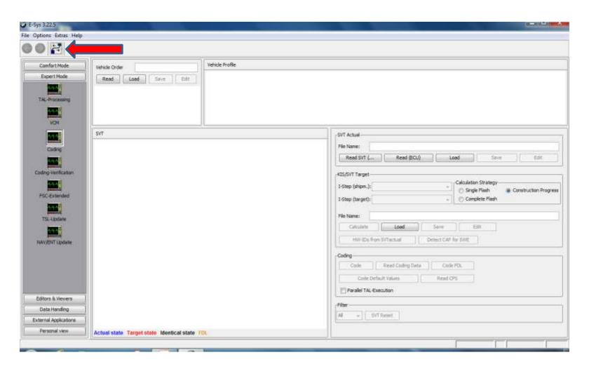
Select the correct TargetSelector, e.g. F010 (not F010\_DIRECT) for an F10 Select "Connection via VIN" and press the "Connect" button. (Ignore the Vehicle-Specific parameter options.) Click OK in the popup box which appear when connection established.
