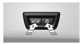
Press the button, arrow 1, on the inside of the tailgate.
