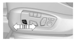
Adjust the position using the lever.
