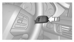
Press the button on the wiper lever.
