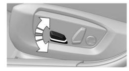
Move the control in the desired direction until the desired tilt is set. After releasing the control, apply your weight to the seat or lift it off to make sure the seat engages properly.
