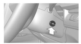
If a corresponding Check Control message appears, hold the remote control vertically against the marked area on the steering column and press the Start/Stop button within 10 seconds while pressing the brake.
