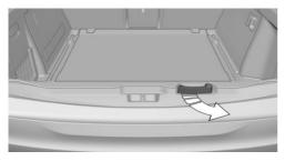
Pull the lever and swing down the tailgate. The open tailgate can be loaded with up to 550 lbs/250 kg.
