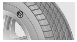
RSC label on the tire sidewall.
