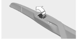
4. Slide wiper blade out of the wiper arm.
