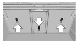
There are three mounting points for the upper retaining strap of LATCH child restraint fixing systems.
