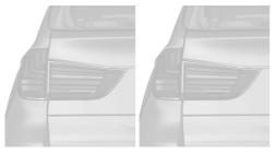
During normal brake application, the outer brake lamps light up. During heavy brake application, the inner brake lamps light up in addition.
