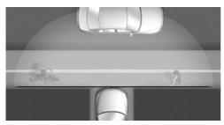
Panorama View provides an early look at cross traffic at blind driveways and intersections. Road users concealed by obstacles to the left and right of the vehicle can only be detected relatively late from the driver's seat. To improve the viewing, each camera, front and rear on the vehicle, detects the traffic area on the side.
