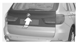
Press the button on the exterior of the tailgate.
