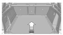
Raise the cargo floor panel. The storage space under the cargo floor panel is subdivided.
