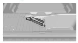
The screw-in tow fitting should always be carried in the vehicle. It can be screwed in at the front or rear of the BMW. It is located in the onboard vehicle tool kit under the cargo area floor.
