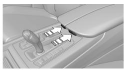
Push the cover down slightly and press the button, see arrow. The respective cover folds up.
