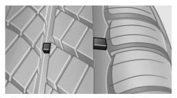
Wear indicators are distributed around the tire's circumference and have the legally required minimum height of 0.063 in/1.6 mm.
