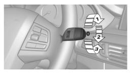
Turn switch from idle position 0 upward, arrow 1: interval mode. When reverse gear is engaged, the system switches to continuous operation.
