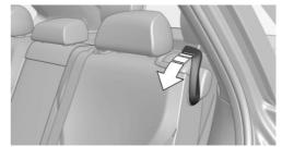
Pull the lever and fold the seat forward.The recessed grip on the inside trim of the door pillar makes getting into the vehicle eas-
