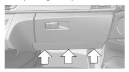
Loosen fasteners, arrows, and open cover.
