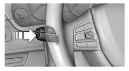
The High-beam Assistant can be activated when the low beams are switched on.
