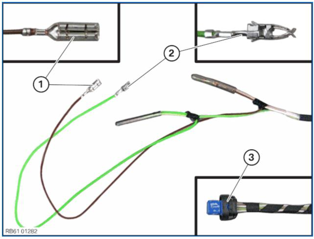
Connect connector (3) with the rear view camera.
