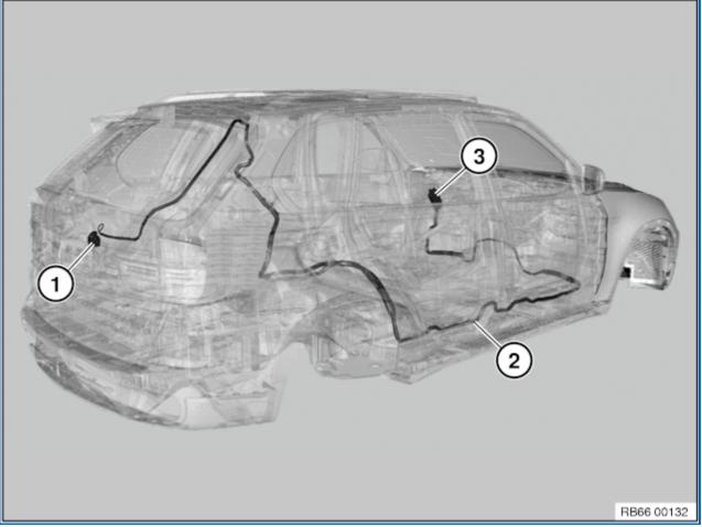
Route repair cable from the rear view camera (1) along the wiring harness (2) to the headunit and attach appropriately.
