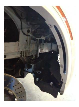
Step 4: Removing the side air vent
