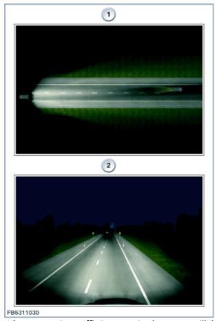
When oncoming traffic is recognised, a range will develop that is only scarcely illuminated by the high-beam headlight. Outside of this range, the optimized illumination of the road will be maintained (1). The non-glare alignment will adjust to the movement of the other road users as needed. When the oncoming vehicle passes an unfavourable angle, the high-beam headlight facing him will be deactivated (2). The high-beam headlight temporarily switches to the dimmed mode.
