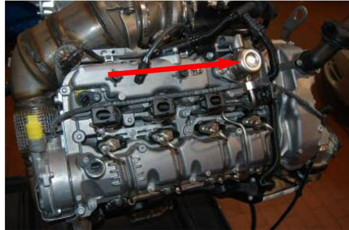
This means the piston is permanently moved by the three-point cam as soon as the engine is running. Fuel therefore continues to be pressurized for as long as new fuel is supplied to the high pressure pump via the volume control valve.
