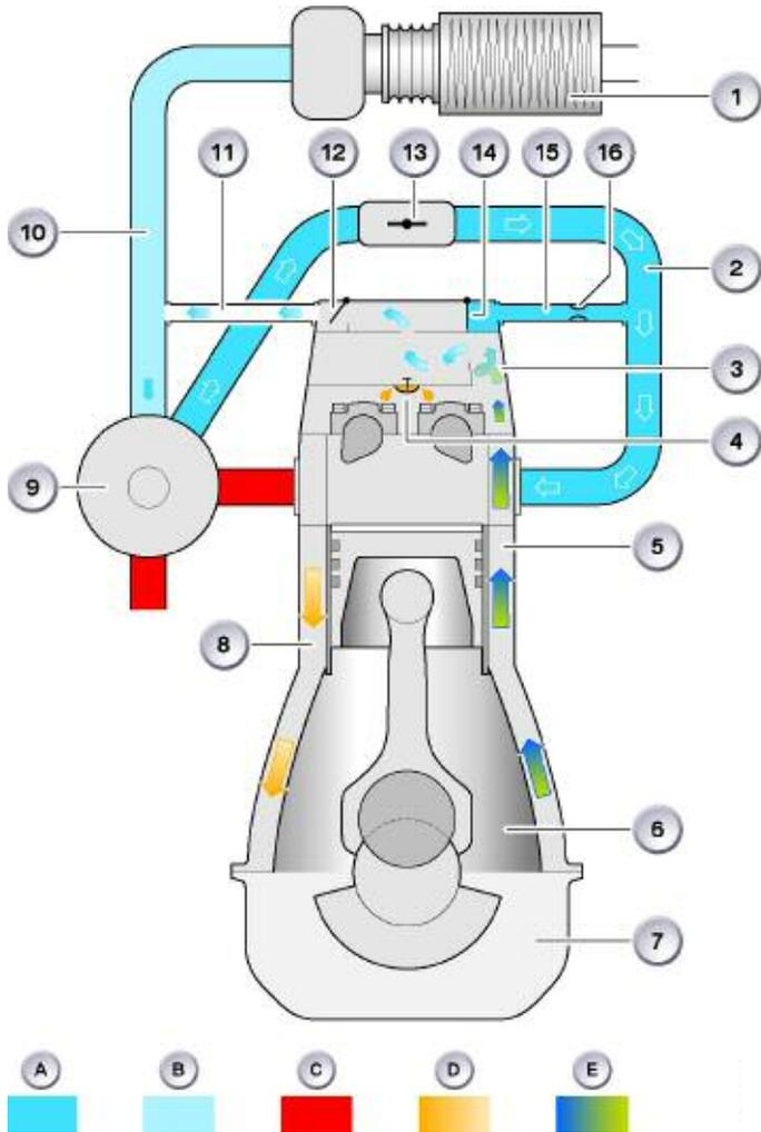
This is realized in the N63 engine with a restrictor, which limits the throughflow and thus also the pressure level in the crankcase breather. As the illustration shows, ventilation takes place during naturally aspirated operation via an external line from the cylinder head cover to the intake manifold.
