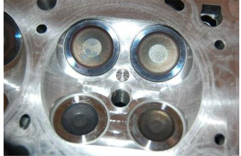
The intake port features a trailing edge for creating more intensive charge movement. The fuel injectors and spark plugs are arranged transversely adjacent to each other in the center of the combustion chamber roof.
