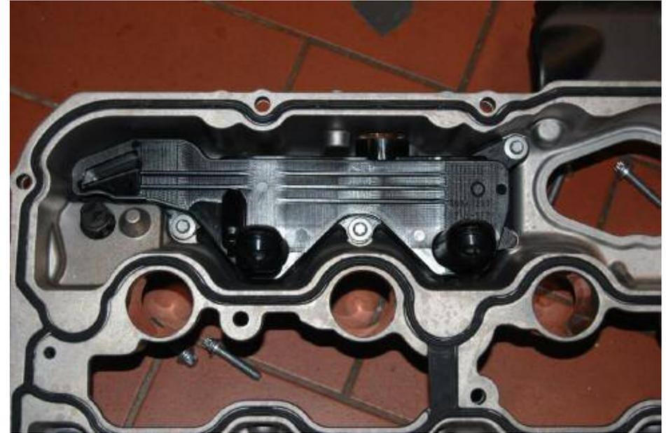
**Note:** If the exhaust system produces blue smoke, it is necessary to check whether the engine is also drawing oil into the combustion chamber through the crankcase breather, which suggest that there is a fault in the area of the crankcase breather. A clear sign of a problem is an oiled up clean-air pipe.
