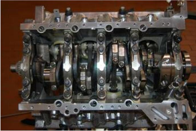
The oil pump on the N63 engine is driven by the crankshaft on the flywheel side. The sprocket is built directly into the crankshaft.
