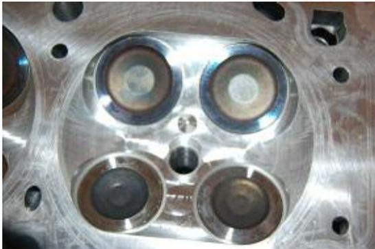
The piezo-injector is integrated together with the spark plug centrally between the inlet and exhaust valves in the cylinder head. This installation position prevents the cylinder walls or the piston crown from being wetted with injected fuel.
