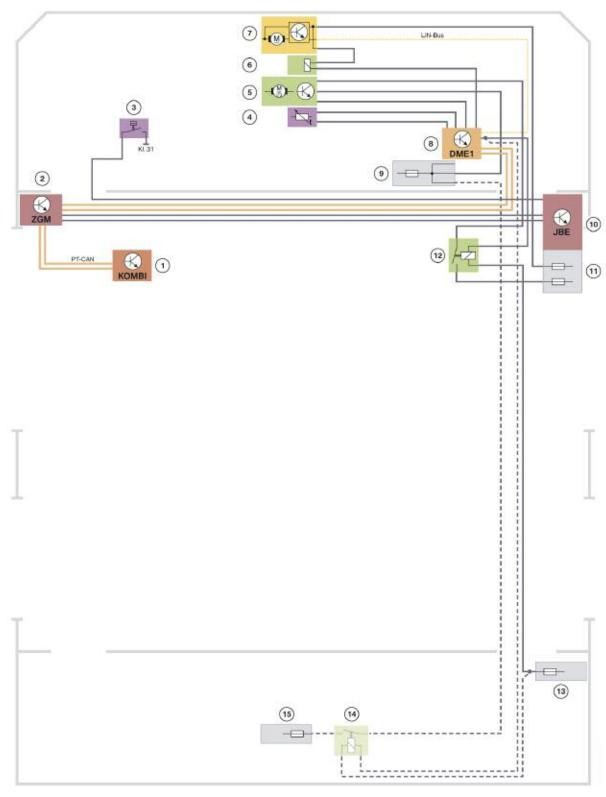
N55, circuit diagram, engine cooling
