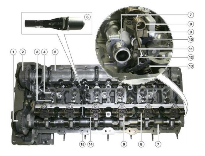
Note: Notice the hollow, lightweight design of the camshafts (7) and the blow-by passages leading into the intake ports (15).
