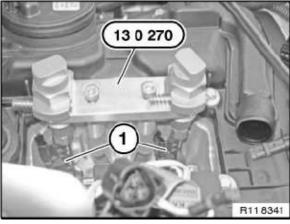
Note: Do not open the high pressure fuel injection system if the coolant temperature is above 40°C. The residual pressure in the high pressure fuel system could cause bodily injury.
