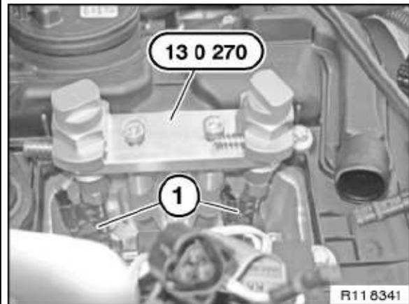
**Note:** Do not open the high pressure fuel injection system if the coolant temperature is above 40°C . The residual pressure in the high pressure fuel system could cause bodily injury.
