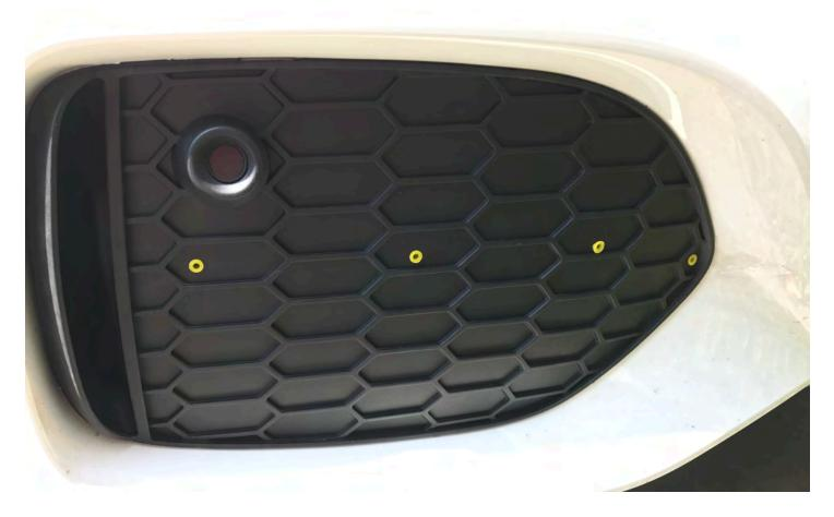
Step 3: Put the back mounting piece against the grill, line up the hole and insert the supplied screws then tighten them using the phillips screwdriver by hand. DO NOT USE POWER TOOL.
