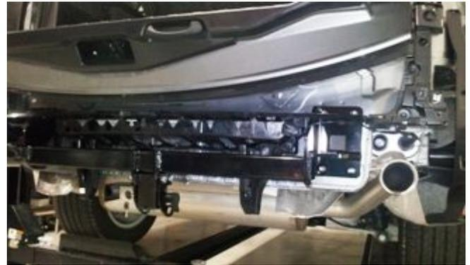
14. If installing a wiring harness, perform all wiring steps now, per the wiring instructions, prior to tightening the hitch beam to the chassis.
