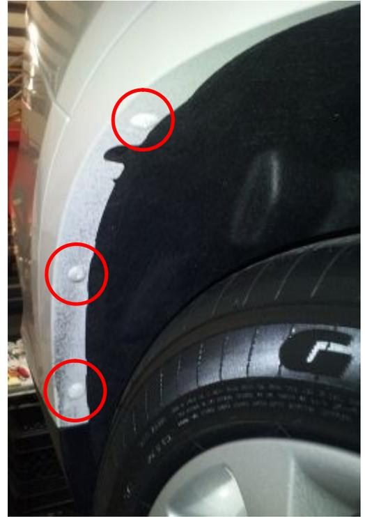
2. Starting at the bottom edge of the fenderwell, use plastic pry tool to carefully unclip fenderwell trim from rear fascia.
