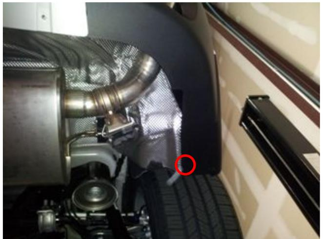
5. While under the vehicle, locate the backside of the reflectors, squeeze the center clip and push. This will partially dislodge the reflectors.
