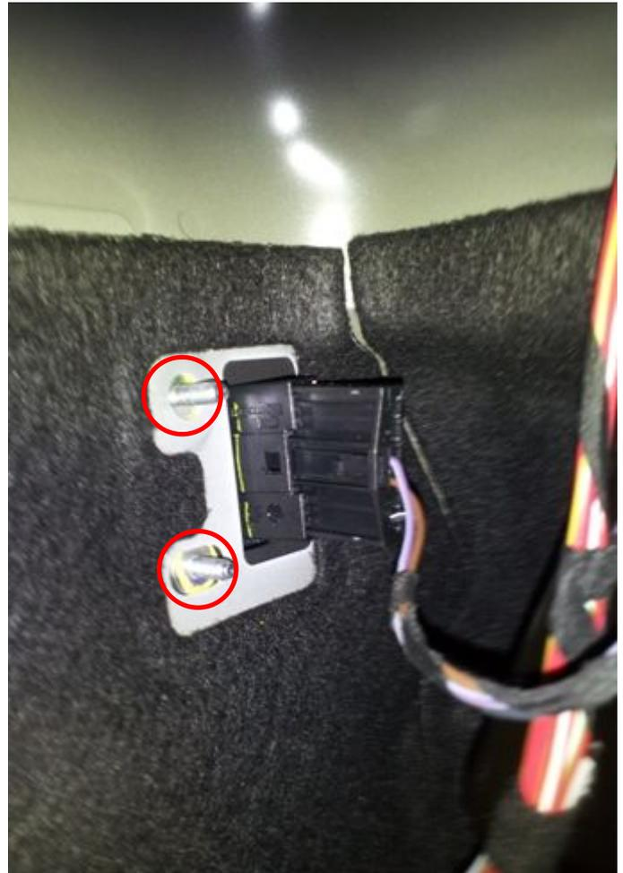
8. Remove hidden, downward screw exposed by taillight removal (1 per side). 8mm socket required.
