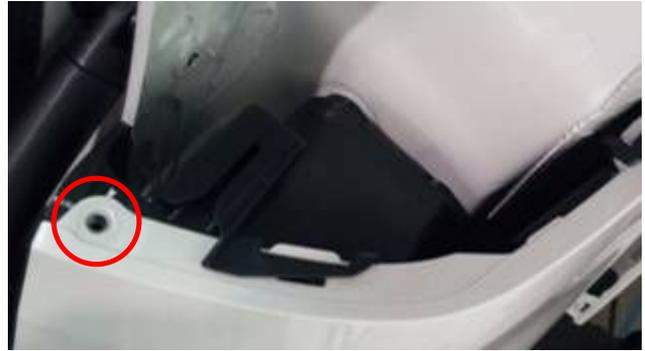
9. Use plastic pry tool to unclip fascia, starting at each fenderwell and working toward the center.
