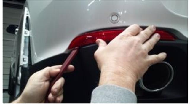
7. Inside the cargo area, remove the Left and Right side panels to expose the back of the tail lights. Then remove the taillight assemblies.
