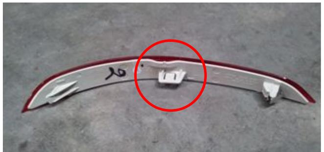
6. From behind the vehicle, pry out reflectors using plastic pry tool at the edge of reflector that is most toward the side of the vehicle. This will expose a hidden screw behind each reflector.
