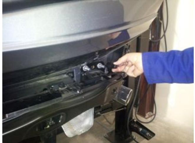
13. Assemble the *invisihitch* latching mechanism onto the hitch beam per the assembly diagram.
