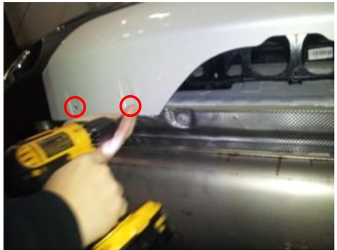
4. Continuing on the underside, remove the screws located near the outer corners of the fascia (1 per side). Requires 8mm socket.
